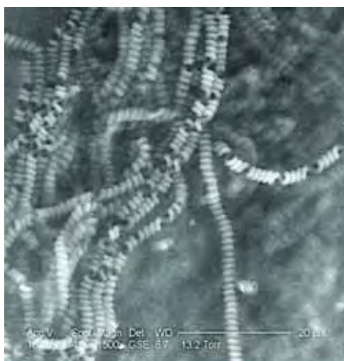
Fig. 3. ESEM micrograph of live cyanobacteria spirulina on agar gel. T = 20^{\circ}\text{C} , p_{H_2O} = 13.2 torr ( \sim 75\% RH). Reproduced, with permission (Stokes, Baker & Toth, 2004). Imaged using an FEI XL30 FEG ESEM. Horizontal field width = 68\ \mu\text{m} .
