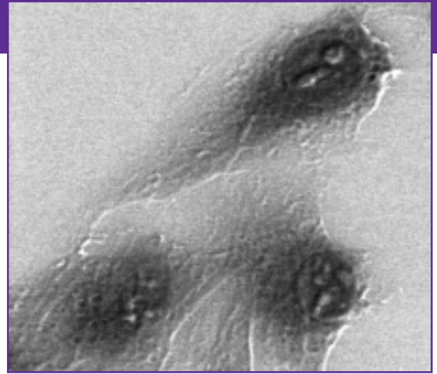
Figure 11: Chemically fixed cells Electroscan 2010, beam energy: 10 keV, total working distance: 8.5 mm, pressure: 2.9 torr, specimen temperature: 3°C, magnification: 750x (horizontal field width: 85 µm)
